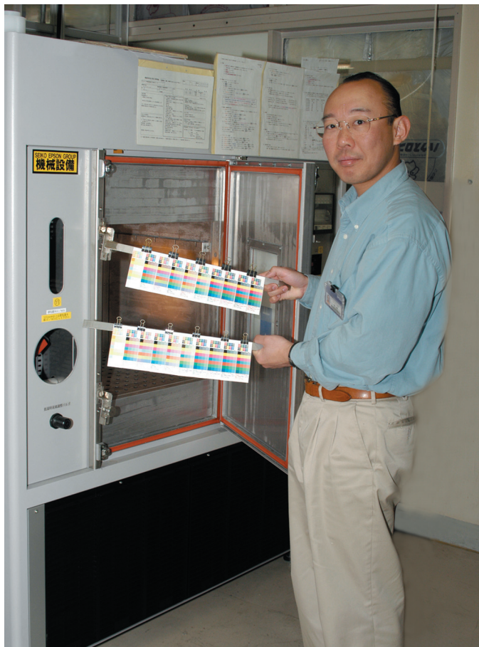
Environmental Testing Chamber, Seiko Epson Corporation
