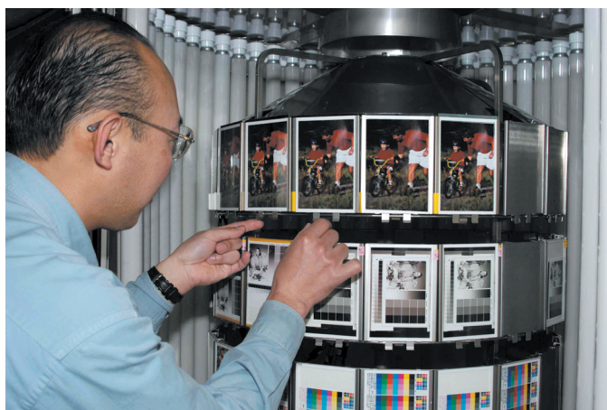
Lightfastness Testing Chamber, Seiko Epson Corporation
