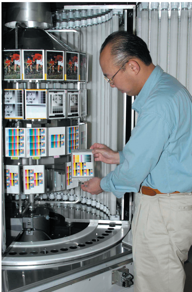
Lightfastness Testing Chamber, Seiko Epson Corporation
